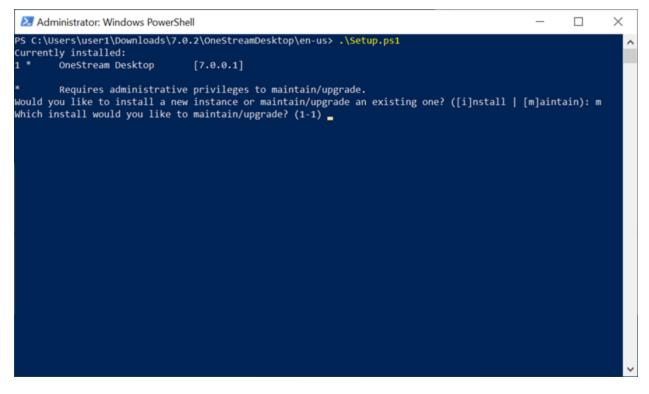
Because the PowerShell is elevated, the existing install can be maintained. Selecting 'i' from the first prompt will install a new per machine instance, while selecting 'm' will prompt you for which instance to maintain, which will then launch the installer for that instance.
